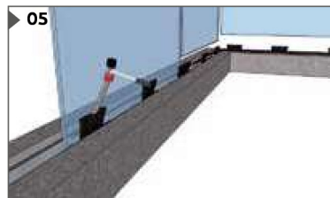
Rest the glass into the block and fixed it with the plastic wedge.
