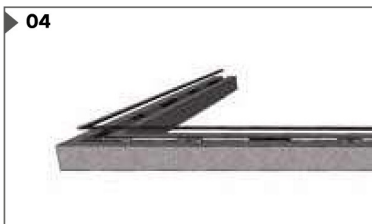
04 Fixed the outside system cover on the outer face of the blocks.
