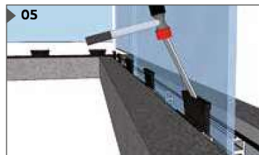
05 Rest the glass into the block and fixed it with the plastic wedge.
